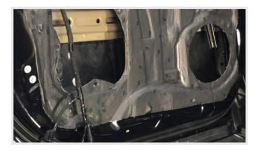
Use **super glue** or **Double Sided Tape** to attach the Speaker Tweakers **directly behind** each speaker on top of the **Damplifier Pro**™.
