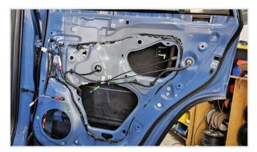
Measure and cut Damplifier Pro™ mats with a utility knife to fit. Use a cardboard template if desired. We recommend **60% coverage** on outer skin and **40% coverage** on inner skin (avoid mechanical and/or electrical components).
